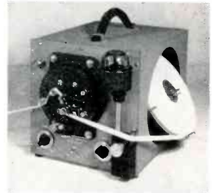
Mecanitron recorder that inks out automatic transmissions at speeds as high as 1200 words per minute
