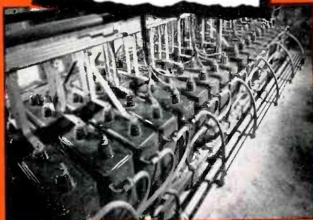
"Made induction heating practical"—This bank of G-E water-cooled capacitors is used with two Ajax-Northrup induction-type steel furnaces in a Western metals plant.
