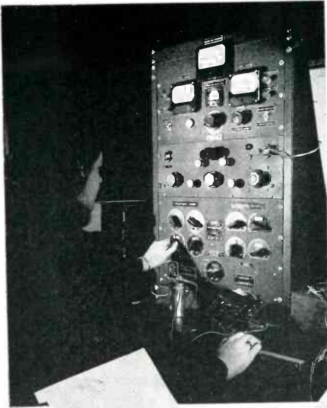
An Aerovox capacitance bridge for measuring capacitance, equivalent series resistance, leakage and other electrical characteristics of electrolytics.
