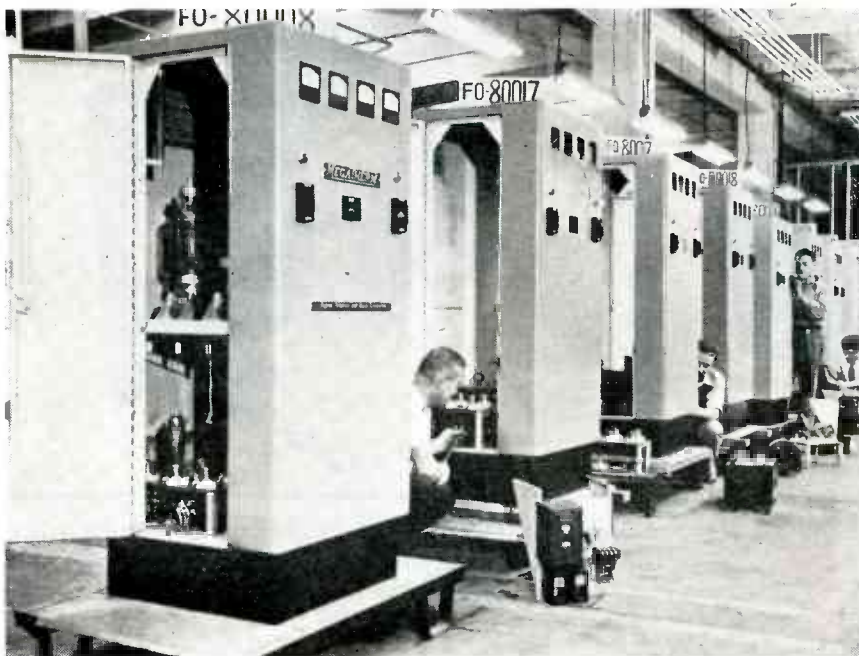
These Megatherm units are built for controlled surface and spot heat treatment in the metal industry and have been used for dielectric heating in the plastics, textile, food and woodworking industries. The assembly-line technique is employed in the plant of the Industrial Electronics Products Division of Federal Tel & Radio Corp.
