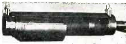
Measuring head in hydraulic-type holder, showing concentric steel shells used for routine calibration and check of performance
