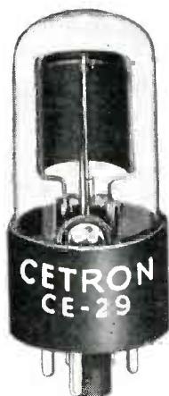
Particularly sensitive to blue and violet light. RMA spectral sensitivity designation S-4. 5-Pin base interchangeable with other similar tubes.
