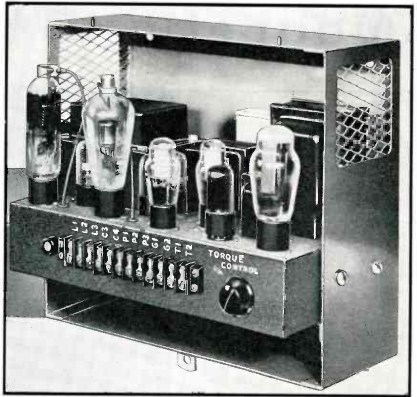
Rear view of chassis using circuit of Fig. 4. This control unit supplies 220 watts of d-c excitation for machines of from 1 to 75 horsepower
