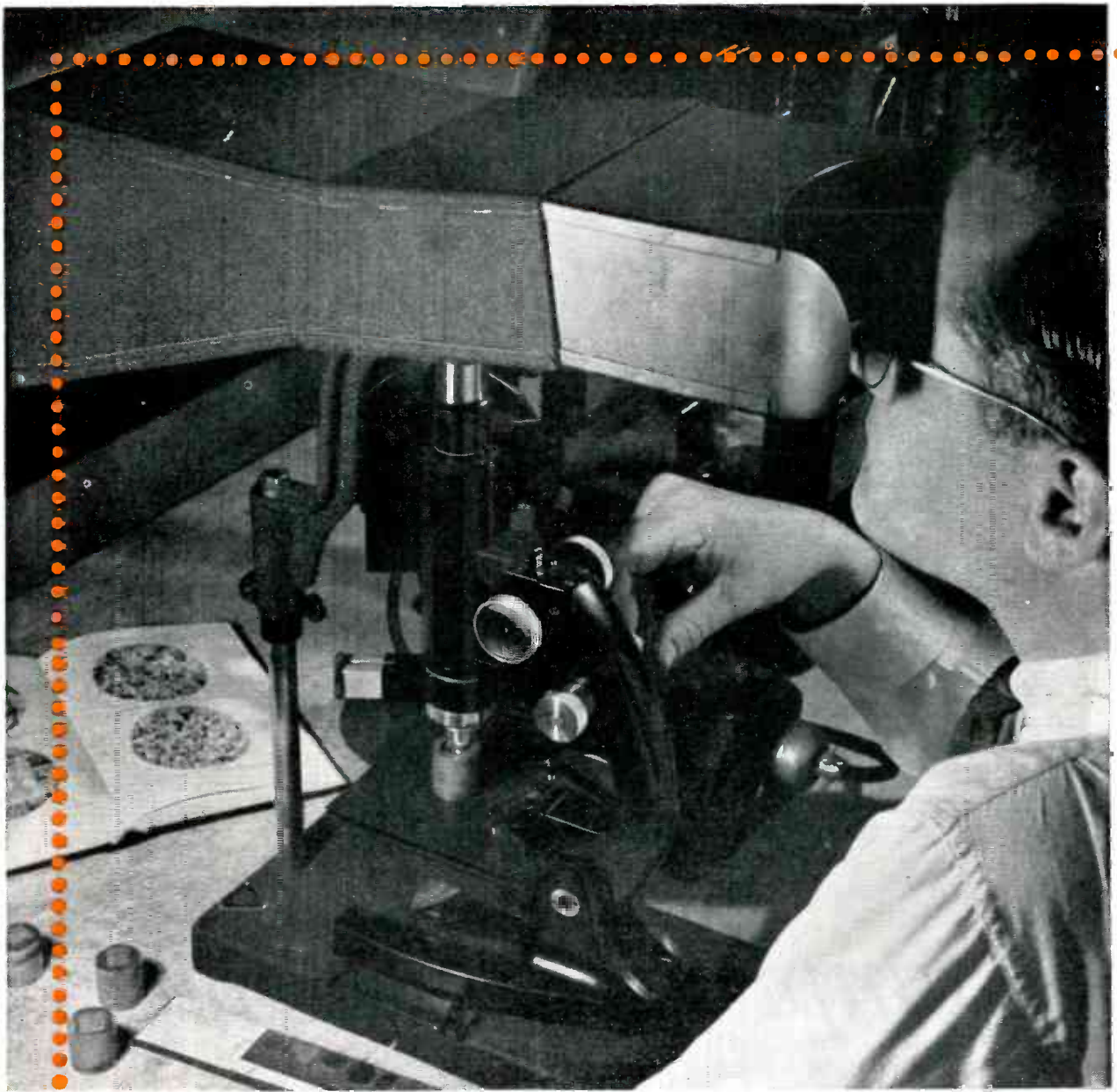
Investigating the grain structure of a metallurgical subject, magnified 585 times.
