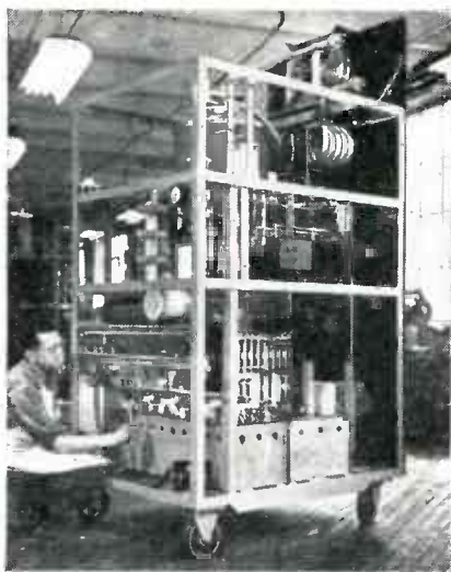
High frequency induction furnace used in all radio tube plants where exhaust machines operate. Made by Sylvania Electric at Williamsport, Pa.
