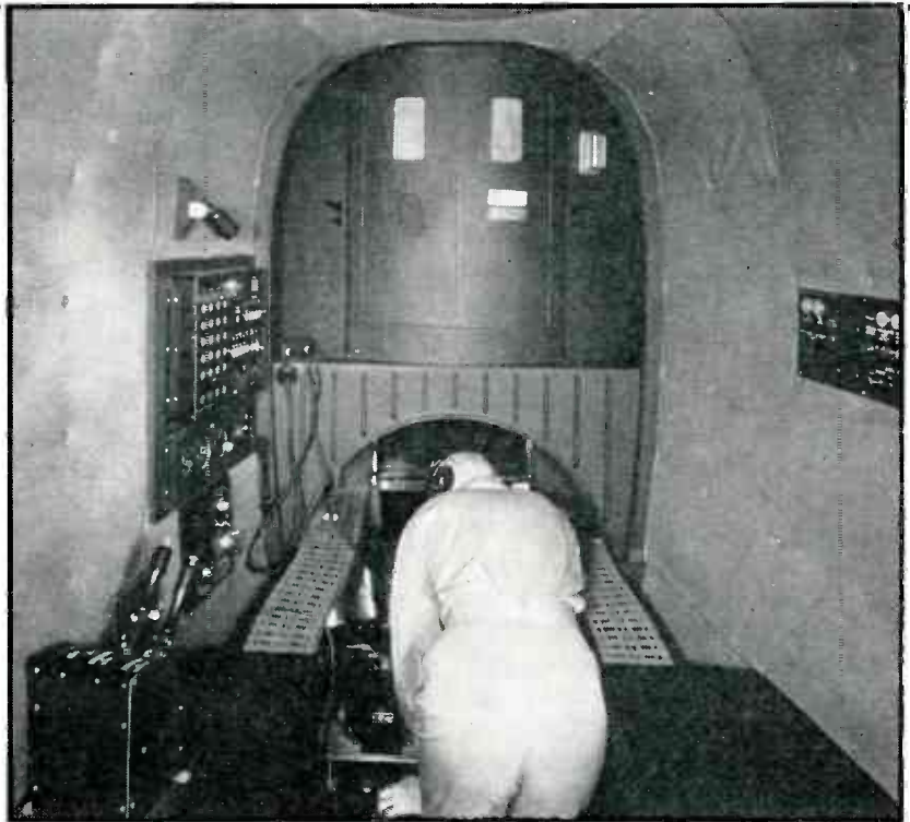
FIG. 1—Interior of the bombardier's compartment in the PB4Y mockup. Two loudspeakers are mounted behind the cloth wall above the bombardier's head and two others are concealed in dummy ammunition boxes at each side
