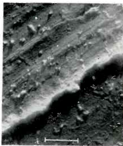
The shadow-cast of a replica of the inner surface of a bearing race shows effects of wear. Scale line represents fifty millionths of an inch
